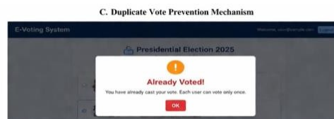
Fig. 3. Duplicate Vote Restriction Alert The system prevents multiple voting by verifying the user's voting status before allowing vote submission.
